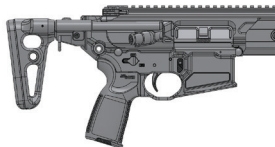
STOCK FULLY COLLAPSED
