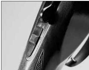
The thumb "safety" shown in the rearward "on safe" position.
