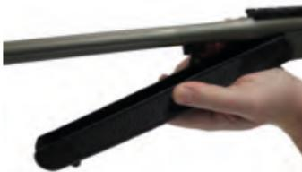
4. Press the barrel catch lever to remove the barrel from the frame.
