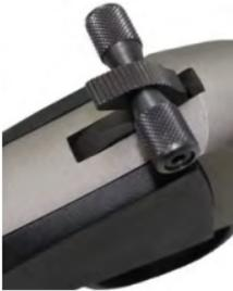
When the hammer is in the **At Rest** position the internal hammer block safety is preventing the hammer from striking the firing pin unless the manual trigger safety is disengaged and the trigger is pulled. Note: There should be a small gap between the hammer and frame in this position.
