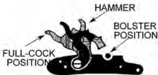
PERCUSSION: EXTERNAL LOCK PARTS
