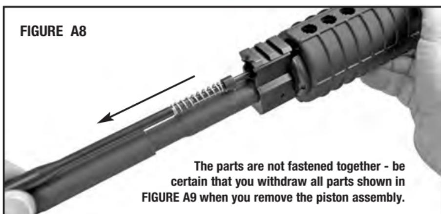
The parts are not fastened together - be certain that you withdraw all parts shown in FIGURE A9 when you remove the piston assembly.
