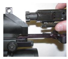
11. Push the charging handle assembly and bolt carrier assembly together into the upper receiver.
