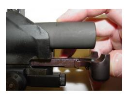
1. Pull back the charging handle and bolt carrier assembly.
