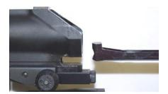
3. Pull the charging handle back aligning the tabs on the charging handle with the cut outs on the inside of the receiver and bring it down to remove it.
