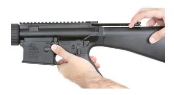
3. Place the safety on "SAFE". Squeeze the trigger. The trigger should not fall.
