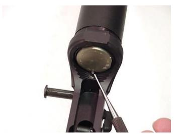
1. Cock the hammer with your thumb. Push in the buffer and depress the buffer detent to release the buffer.
