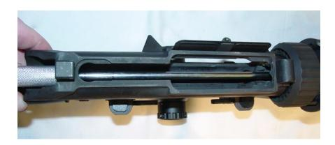
2. Install the chamber brush on the cleaning rod, dip it in cleaning solvent, and insert it into the chamber and locking lugs. Clean by pushing and twisting the cleaning rod.
