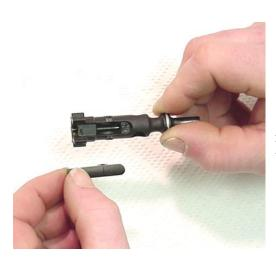
11. Remove the extractor and spring assembly. Do not remove the spring assembly, its insert or the O-ring from the extractor unless it needs to be replaced.
