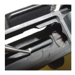
3. Use a worn out bore brush to clean the outside surface of the protruding gas tube (get the sides and bottom from the bottom of the upper receiver). This procedure ruins the brush for bore cleaning.
