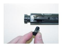
6. Drop the firing pin into its opening.
