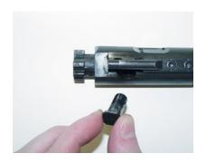
7.Lift out the cam pin.
