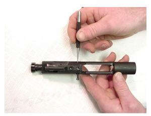
4. Move the bolt assembly forward to the unlocked position and remove the firing pin retaining pin. This can be done by either pushing it from right to left with a pin punch or pulling it from the "loop" side. Do not open or close the split end of the firing pin retaining pin.
