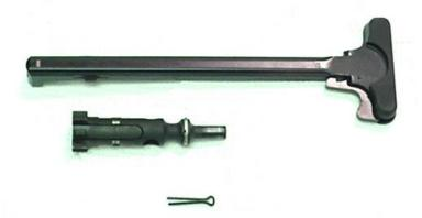
7. Inspect the bolt assembly for cracks or fractures, especially in the cam pin hole area.
