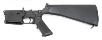
3. Clean the buffer, operating spring, and inside lower receiver with a swab dipped in solvent.
