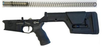
2. Remove the buffer and the operating spring
