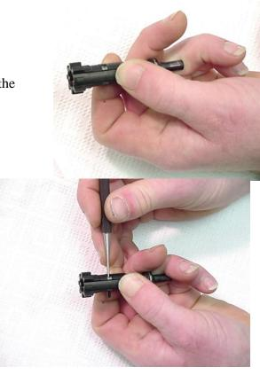
10. Use a punch or dummy round to remove the extractor pin.
