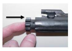
5. Push in on the bolt assembly to put it in the locked position.
