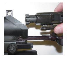
2. With the charging handle approximately half way to the rear you can remove the bolt carrier assembly. Remove the bolt carrier assembly.
