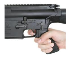
4. Place the safety on "FIRE". Squeeze the trigger and hold the trigger to the rear; *the hammer should fall*. Pull the charging handle to the rear and release it. Release the trigger. *You should hear a click as you release the trigger*. Squeeze again; *the hammer should fall*.
