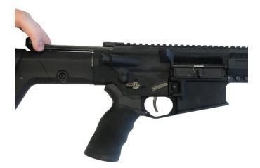
2. Push the magazine up into the receiver until the magazine catch engages and holds the magazine.
