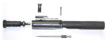
1. Clean all parts and outer surfaces of the bolt carrier assembly with a swab saturated with cleaning solvent.
