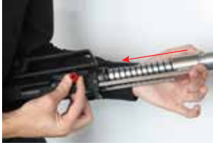
Photo 13-) Pull the action bar until the charging handle and the hole (charging handle lock hole) is parallel for unlocking the charging handle of F12. Then pull the charging handle to right side of the gun for disassembling charging handle.
