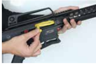
Photo 2-) Pull F12 charging handle to operation direction then use shell safety kit (yellow part) to make ready your gun disassembling in right way. If you do not use that shell safety kit, you will damage shell carrier ramp absolutely!!!
