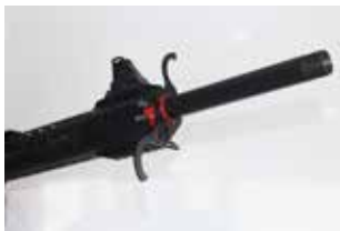
Photo 9-) Use your F12 Special Wrench Set for starting to disassemble forend of your shotgun.
