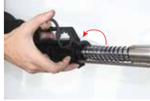
Photo 14-) Use your F12 Special Wrench Set for turning the barrel nut of your gun.
