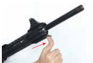
Photo 10-) Pull or push sling swivel apparatus to the thread of barrel for passing next step.
