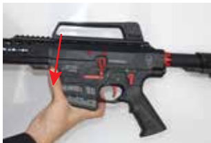
Photo 7-) Push pivot pin at the front sight of lower frame by a tool or your finger as in the photo.
