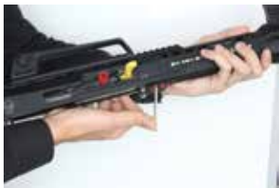
Photo 11-) Use the 4.00 mm allen wrench in your F12 tool set for turning the screws on bottom side of forend for starting to disassemble forend of your shotgun.
