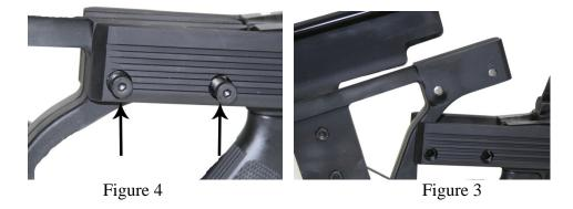
Push the buttstock (S-9) up and forward to install it on the forestock (S-1) (See Figure 3). Install the two buttstock screws (S-2) at the right rear of the forestock using a 5/32 inch Allen wrench (See Figure 4).
