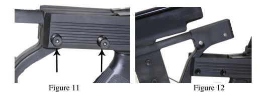
6. To remove the buttstock (S-9) from the forestock (S-1), remove the two buttstock screws (S-2) at the right rear of the forestock using a 5/32 inch Allen wrench (See Figure 11). Pull the buttstock down and to the rear to remove it (See Figure 12).
