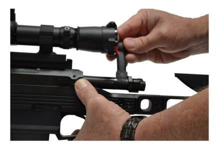
Removing the Bolt Assembly
