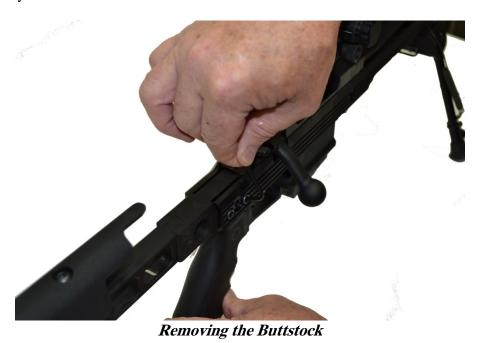
4. Remove the buttstock assembly (A-3) from the forestock assembly (A-2). Remove the two buttstock screws (F-15) at the right rear of the forestock using a 3/16 inch Allen wrench. Pull the buttstock down and to the rear to remove it.
