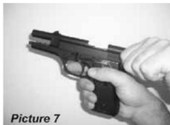
While drawing the slide back, check whether the slide moves easily on the
