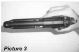
your fingers off the trigger. Check the loaded chamber indicator (PICTURE 3) to see if it is loaded or unloaded.
