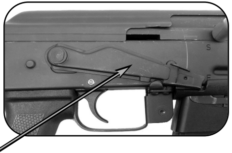
Safety lever in lower or “FIRE” position. Pulling the trigger when the safety lever is in the lower position will result in the rifle firing if there is a round in the chamber! Exercise extreme caution when handling rifle in this condition.
