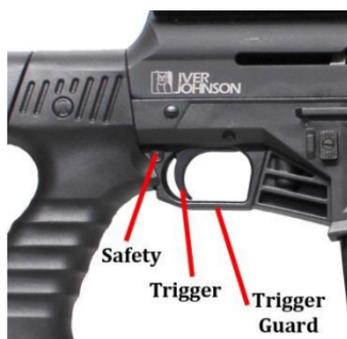
Once the shotgun is loaded, one pull of the trigger will fire one shotshell. After firing, the spent shell will eject, and the next shell will load automatically, making it ready to fire with another trigger pull. See “Firing your Shotgun” for further instruction.
