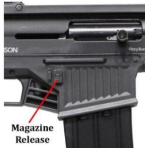
3. Pull the charging handle fully rearward and depress the bolt release latch to lock open the bolt. This will eject a loaded shotshell if there is one in the chamber.
