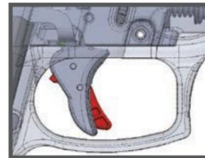
**4. Trigger Safety.** The trigger safety's purpose is to prevent the trigger mechanism from being actuated in the event the firearm was accidentally dropped in certain orientations. Once you are ready to fire and depress the trigger, the trigger safety will automatically move to the fire position.
