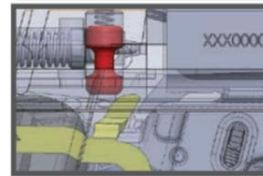
**5. Firing Pin Block.** The firing pin block's purpose is to prevent the gun from firing in the event the firearm was accidentally dropped in certain orientations. The Firing Pin Block interferes with the forward travel of the firing pin until the trigger is pulled. Once you are ready to fire, pressing the trigger moves this safety component from its "safe" (blocking) position to its "fire" (free) position.
