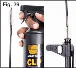
block do not normally need to be cleaned as often as the bore and other action parts. They are considered to be low-maintenance and somewhat 'self cleaning'. They may be cleaned occasionally however to remove any potential carbon build-up or debris. A regular cleaning schedule for these parts may be more necessary if you shoot corrosive ammo, which can create damage through the resulting chemical salt residue.
