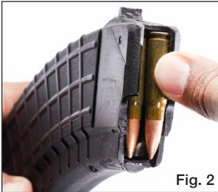
**1.** Load the magazine with the correct ammunition by pressing cartridges one at a time down under the feed lips, ensuring that they contact the rear wall of the magazine. The cartridges will automatically alternate side-to-side. (Fig. 2) It is generally good practice to gently tap the magazine against your palm occasionally to better seat the cartridges and help optimize feeding.
