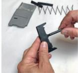
5. CAREFULLY allow the spring to expand. 6. Screw the restrictor into the follower, and
