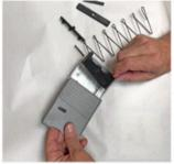
Remove spring and base plates. Separate the reassemble. halves of the magazine enough to allow you to extract the follower.
