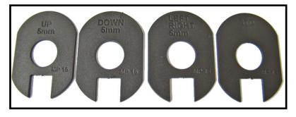
You will probably find that your gun fits comfortably with no adjustment, but if you wish to fine-tune the fit, you may purchase shims from our online store at www.trimports.com. Markings for the adjusting shims are self-explanatory. For RH cast, mount the shim on the receiver so that the printing is visible. Simply reverse for a LH cast. A standard shim provides additional shock absorption.
