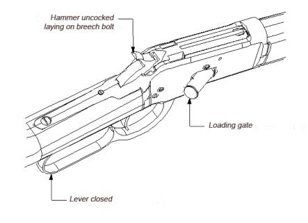
Press the loading gate inward with the tip of the first cartridge until all but the rim has entered the loading gate, then insert the next cartridge in the same manner, pushing the preceding cartridge into the magazine.
