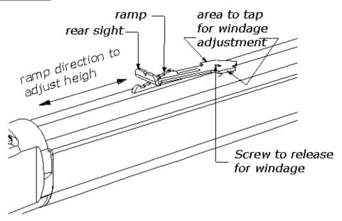
Take a non-marking brass, plastic or fiber hammer and gently tap the rear sight base to the left or to the right according to the direction you wish to move the point of aim. Tighten the screw again.
