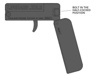
It is highly recommended that the pistol be kept in this half-cocked position whenever it is not being fired. The pistol must be placed in the half-cocked position for loading and unloading. NEVER ATTEMPT TO LOAD THE PISTOL WITH THE BOLT COCKED! In the half-cocked position, the bolt is captured and the trigger cannot be pulled. Do not carry the pistol with a live cartridge in the chamber.
