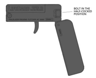
Slide the barrel release latch fully rearward and lift up on the barrel.
