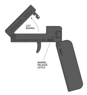
Place the proper ammunition into the chamber and ensure that it is seated fully.
