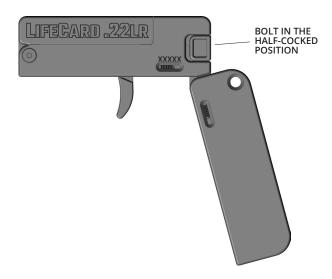
It is highly recommended that the pistol be kept in this half-cocked position whenever it is not being fired. The pistol must be placed in the half-cocked position for loading and unloading. NEVER ATTEMPT TO LOAD THE PISTOL WITH THE BOLT COCKED! In the half-cocked position, the bolt is captured and the trigger cannot be pulled. Do not carry the pistol with a live cartridge in the chamber.
