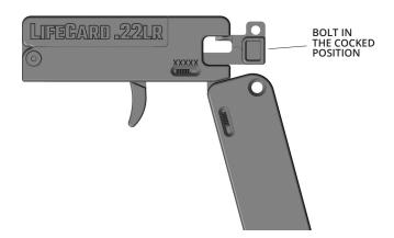
Aim at the intended target and pull the trigger fully rearward. After firing always return the bolt to the half-cocked position by firmly grasping the recessed sides of the bolt and drawing it slightly rearward until it aligns with the rear of the frame.
