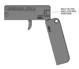
Slide the barrel release latch fully rearward and lift up on the barrel.
