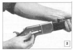
When loading cartridges through the ladle, leave the rim of each cartridge protruding sufficiently to hold the ladle open.
