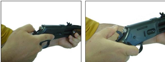
When cartridges no longer eject, open the action of your rifle and visually check the chamber and feed ramp as well as the magazine mechanism for cartridges.
