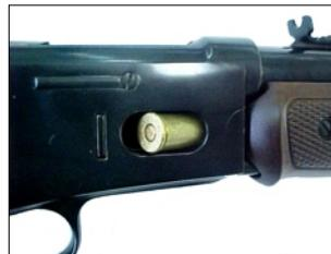
2) Insert the next cartridge in the same manner, pushing the preceding cartridge into the tubular magazine.
