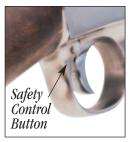
The Taurus Model 63 Rifle is equipped with a cross bolt type safety. The safety control is located on the rear of the trigger guard. The control is a button that can be operated easily with gloved hands as well as barehanded. When the safety is in the "ON" or "Safe" position, the trigger is blocked from movement and the rifle cannot be fired with a normal trigger pull. It is essential to safe shooting that you become
