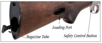
Twist the end of the magazine tube approximately 1/8 turn counter-clockwise to unlock. Slowly pull the tube out, observing the loading port on the right side of the stock. Pull the magazine tube out until the magazine follower at the end is clear of the loading port. Do not completely remove the tube from the stock
