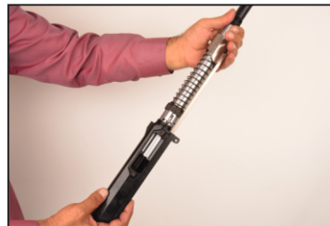
11) Separate the Barrel from the Upper Receiver
