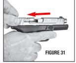
Lock the slide in the open position by allowing the slide to move slightly forward from the rearmost position while pressing upward on the slide stop (FIGURE 32).
