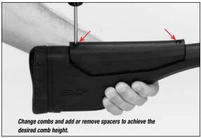
electronic or optical sights. The comb height is adjusted by installing one of the included combs and, if necessary, adding or removing the included spacers. Comb height can be raised a maximum of 1-1/4" when the tall comb is installed in conjunction with four spacers. Adding one spacer will raise the comb 1/8"; a maximum of two spacers per side can be added.
