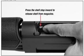
stop, located on the inside-right of the ejection port, to release a shell from the magazine (Figure 12, page 21). Press the shell stop again to release the next shell.
