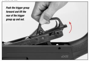
The trigger group should be removed before you attempt to remove the bolt assembly.
