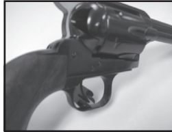
TRIGGER BLOCK FULLY INSERTED
