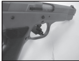
TRIGGER BLOCK FULLY INSERTED
