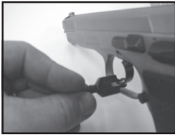
TRIGGER BLOCK BEING INSERTED
