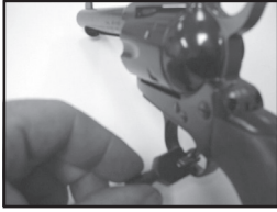
TRIGGER BLOCK BEING INSERTED
