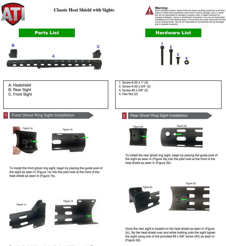
Once the front sight is seated on the heat shield as seen in (Figure 1c), flip the heat shield over and while holding onto the sight tighen the sight using one of the provided #6 x 3/8" screw (#3) as seen in (Figure 1d).
