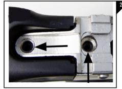
With the pivot housing assembly in the receiver, mark the two holes using a pen as seen in Figure 2. Measure the outside of the screw to make sure it measures .230". If the screw you are using does not have an outside diameter of .230", measure the outside diameter and use the appropriate drill bit.
