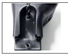
If the screw measures .230 remove the pivot assembly and start by drilling pilot holes in the center of the 2 marked holes with a 1/16" starter drill bit as seen in Figure 3. Next, move up to the 3/16" drill bit and drill 2 wider holes using the two pilot holes.
