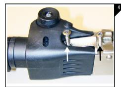
Place the pivot housing assembly into the receiver, insert the (2) original screws and tighten both screws to secure the stock to the receiver as seen in Figure 4.
