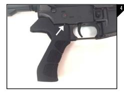
Insert the safety selector spring into the designed hole on the ATI AR-15 X2 pistol grip. Next, slide the pistol grip into place as seen in Figure 4.
