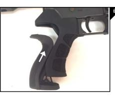
Re-install the Scorpion Recoil Pad by sliding it upward into the pistol grip as seen in Figure 6.
