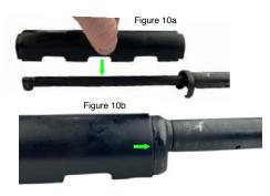
To install the gas tube cover onto the gas tube, begin by placing the cover as seen in (Figure 10a) onto the gas tube and sliding into place until the front of the handguard is seated as seen in (Figure 10b). Note: Because the SKS is a mil surplus firearm, the band as seen in Figure 10b may be disformed from previous re-manfucturing. Because of this you may need to re-form the band to help with seating of ATI gas tube cover.
