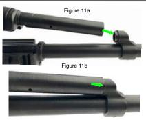
To install the gas tube, begin by inserting the front of the gas tube assembly as seen in (Figure 11a) into the proper location until seated as seen in (Figure 11b).
