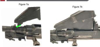
Begin by turning the barreled action over and installing the magazine, making sure to the mate the magazine to the slot on the bottom of the rear sight base as seen in (Figure 7a) until seated as seen in (Figure 7b).
