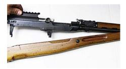
To remove the barrelled action from the stock body, pull outward and towards the rear as seen in (Flgure 2a).
