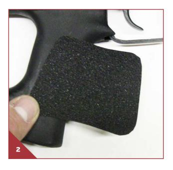
Continue to align the pad to the stock. Keep slight tension on the pad and bring the the pad around the surface of the stock as seen in Figure 3.
