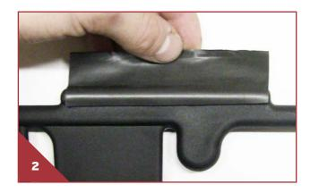
Continue to align the pad to the stock. Keep slight tension on the pad and bring the pad around the surface of the stock as seen in Figure 3.
