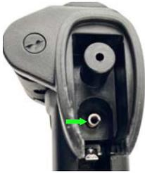
Due to the many variations of the SKS a trigger group spring is required (#2). Insert the trigger group spring into the pilot hole of the grip as seen in (Figure 12a). Installation of the spring will provide a tight fit between the receiver, trigger assembly and Strikeforce Stock.
