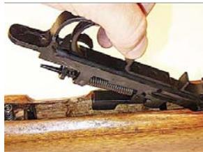
To remove the trigger assembly, begin by inserting a pin punch or phillips head screwdriver into the spring latch catch at the rear of the trigger guard and pressing inward firmly until the spring latch as seen in (Figure 1a). The trigger assembly will now spring out and can be removed from the stock by pulling outward on the rear of the receiver as seen in (Figure 1b).
