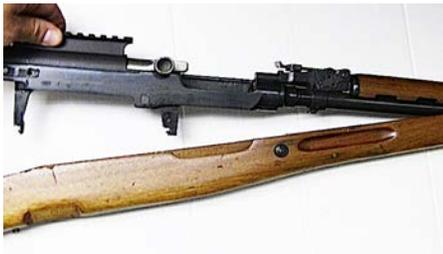
To remove the barrelled action from the stock body, pull outward and towards the rear as seen in (Figure 2a).
