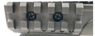
To install the side rails begin by locating the existing pockets on the inside of the stock body and insert (2) 6-32 hex nuts (#7) into the pockets as seen in (Figure 6g). Align the side rail into place and while holding a finger over the hex nuts use a phillips head screwdriver to the fasten (2) 6-32 x 3/8 machine screws (#5) to the picatinny rail as seen in (Figure 6h).
