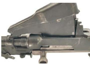
Begin by turning the barreled action over and installing the magazine, making sure to mate the magazine to the slot on the bottom of the rear sight base as seen in (Figure 7a) until seated as seen in (Figure 7b).
