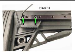
Using the provided (2) 6-32 x 7/16 flat head cap screws (#1) and a 5/64 allen wrench, tighten the shell carrier to the cheekrest as seen in (Figure 1d).
