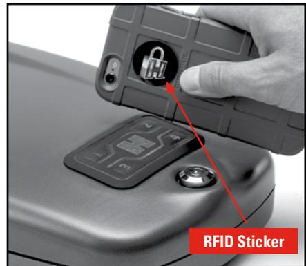
**NOTE:** *The RFID decal can be placed on a variety of objects. However, metal surfaces may cause interference and reduce the read distance. The integrated metal housing on some cell phones combined with potential interference from other wireless signals such as Bluetooth, NFC, etc., may reduce the read distance of the RFID decal.*
