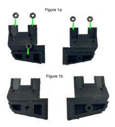
Begin by placing the (5) 6-32 hex nuts as seen in (Figure 1a) into the slots of the cheekrest mounts until seated as seen in (Figure 1b).
