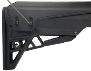
Using the provided 6-32 x 1/4" screws (2) and the appropriate allen wrench, tighten the left side of the cheekrest as seen in (Figure 3c). Turn the stock over and repeat the process to tighten the ride side of the cheekrest as seen in (Figure 3d).
