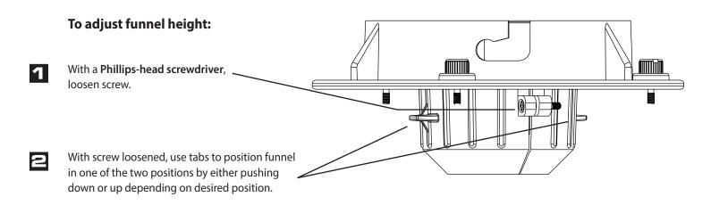
Once the funnel is in desired position, 3 retighten the screw with Phillips-head screwdriver. Do not overtighten.
