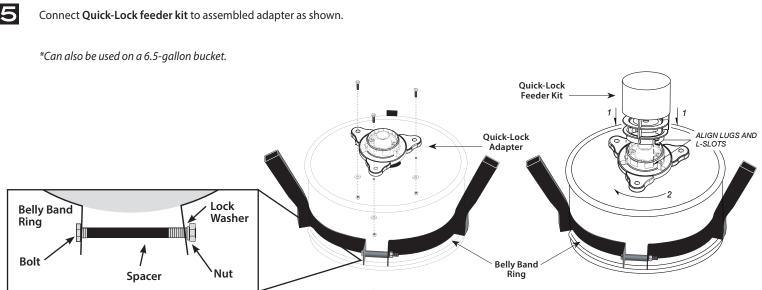
**DO NOT EXCEED 200 LBS DO NOT EXCEED 400 LBS** OF FEED IN 30-GAL FEEDERS OF FEED IN 55-GAL FEEDERS
