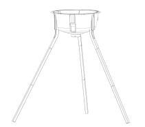
Align holes of hopper top, then press sides of hopper bottom until it snaps snugly in place. Insert bolt through each hole, place lock washer on bolt and screw wingnut onto bolt until tight. Repeat for all 12 bolts.
