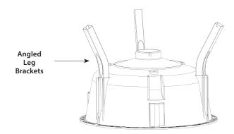
Insert two (2) leg sections into each of the square leg brackets.
