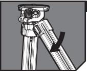
With the MOE Bipod firmly installed, pull the Bipod Legs down until the detents are bypassed and the legs lock into the deployed position at 90 degrees.
