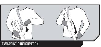
Take the QD Swivel, and depress button to detach. Move the QD Swivel out to the fore-end mounting point of choice on your rail system and attach.
