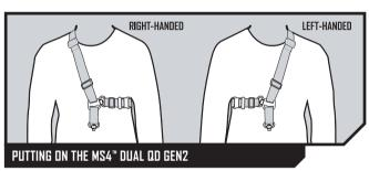
For right-handed users, place your left arm and head through the sling ensuring the *QD Swivel* is oriented forward and the *MST Slider* is located under the left arm. Left-handed users place the right arm and head through the sling, with *MS1 Slider* located under the right arm.
