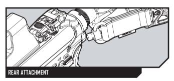
Depress the QD Swivel Button and push the QD Swivel into the QD attachment point on the weapon.
