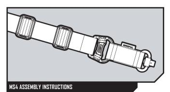
To connect the adapter to the sling, run the tail end (the end of the sling with two Fit Buckles) of the MS1 through the D-Ring on the MS1 MS4 Adapter and then back through the Fit Buckles. Double the webbing back
