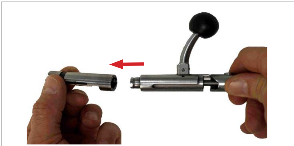
Fig. 16 Pulling off the bolt head
