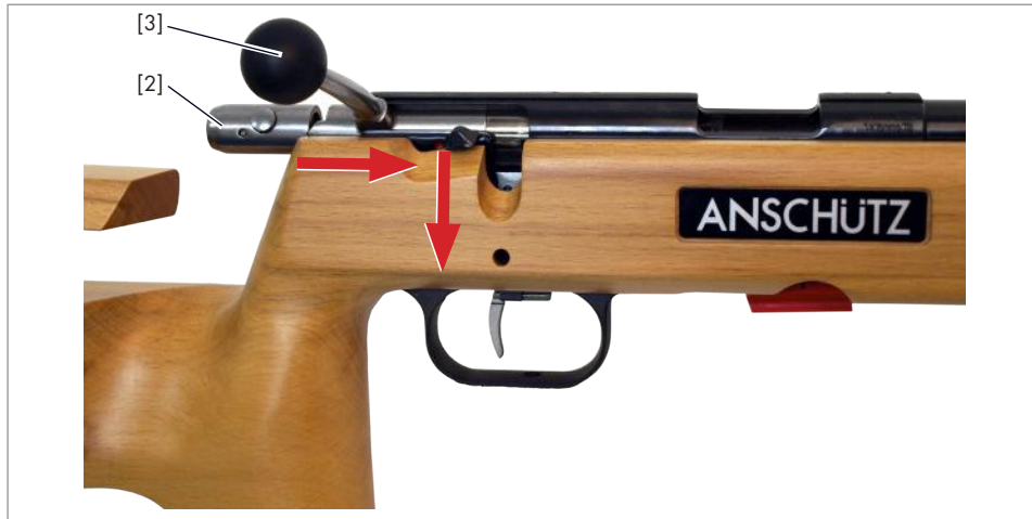
Fig.4 Closing the breech
