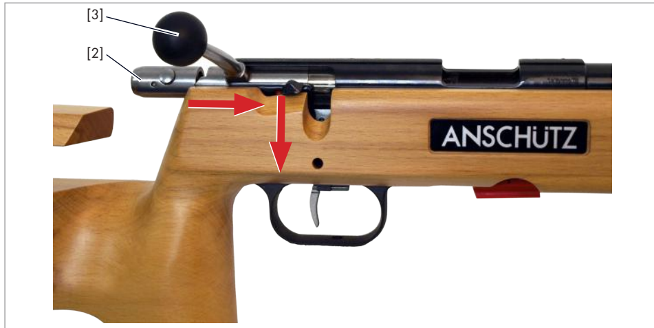
Fig.6 Closing the breech
