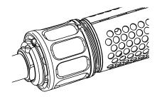
5 Hand-tighten the screw latch, in line with the interior of the muzzle device.
