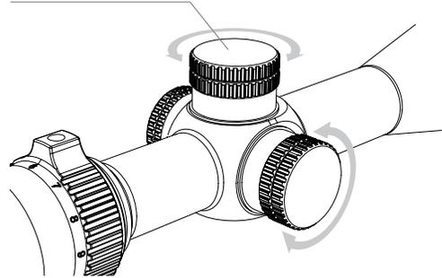
Athlon Neos scopes have 1/4 MOA for the click values of elevation and windage adjustment depending on different configurations of scopes and reticle selections. MOA, a unit of angular measurement, is defined as a minute of angle, a minute is 1/60th of one degree and 1/21600th of a circle. One MOA equals 1.047-inch (rounded down to one inch) at 100 yards, two inches at 200 yards and to ten inches
