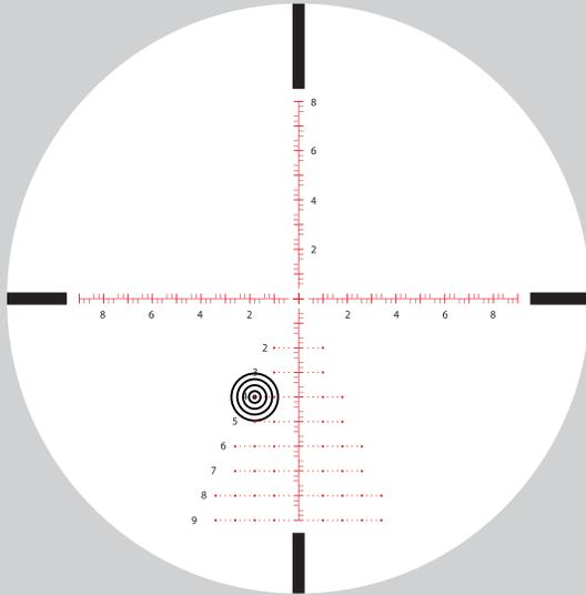
*Use 4 mil to compensate a 86.4 inch bullet drop for a target @ 600 yards, 2 mil wind correction for 15 mph wind from right to left.*
