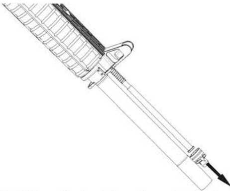
Fig. 15 Removing the piston, piston rod and spring
