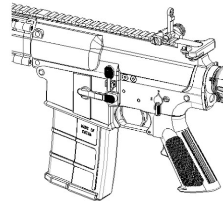
Fig. 4 Removing the magazine by pressing the left hand lock
