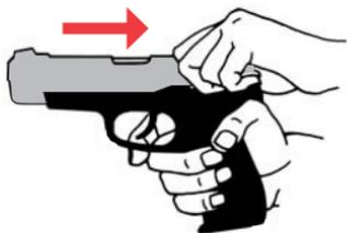
The slide should always be pulled rearward (“retracted”) by pulling the rear portion of the slide in the vicinity of the safety, the decock-only lever, or the serrations (depending upon model). **Always keep fingers away from trigger!**
