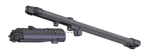
10. Pull the firing pin retaining pin out until it is stopped by its detent.
