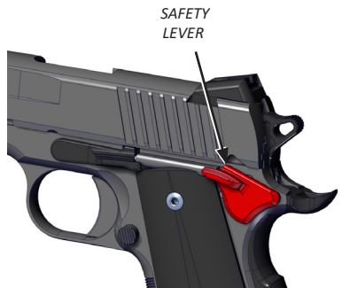
MANUAL SAFETY DISENGAGED (LEFT SIDE)
