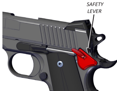
MANUAL SAFETY ENGAGED (LEFT SIDE)
