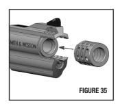
2. Rotate the compensator with your fingers either left or right so that the notch is facing down (in the 6 o'clock position) (FIGURE 36).
